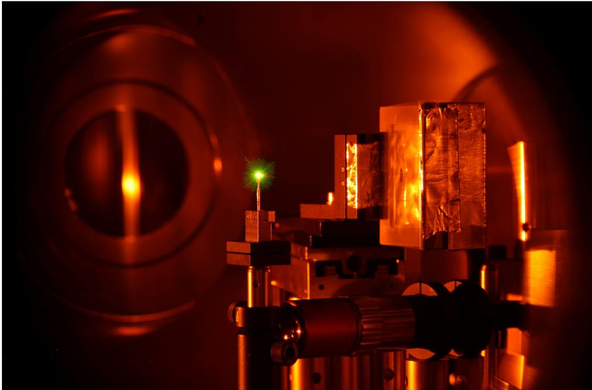
A material sample is placed in the target chamber of GSI's high-performance laser PHELIX. With the aid of the high-intensity laser beam protons are then accelerated out of its back-surface.
